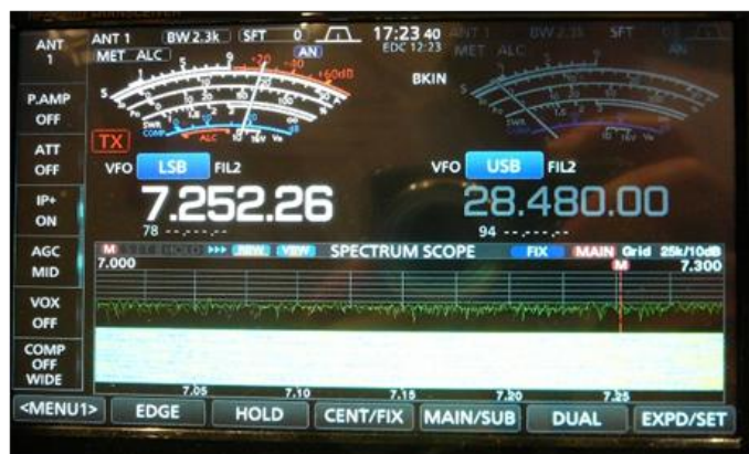
With the Anhtczyk Charger connected my noise level is now S9 +20 db !!!!.
